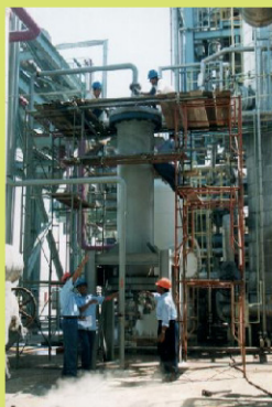
Fig. 2 Reactor in an ammonia plant (PT PIM) containing PIMIT B1 adsorbent.
