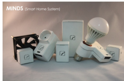
Fig.2 Meshed and Internet Networked Devices System (MINDS) is an Internet-of-Things based system, which connects, controls and monitors all of your home appliances anytime from anywhere.
